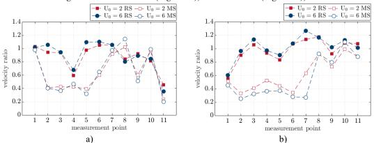
Figure 3. Velocity ratios calculated from the measurements at 1.5 m high, at the different measurement points, for the reference and the mitigation scenarios, for an inflow wind blowing a) from north-northwest and b) from south.
