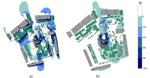
Figure 2. Horizontal iso-contour plots at 1.5 m high, for an inflow wind speed of 6 m.s<sup>-1</sup>. Differences between the mitigation and the reference scenarios for a wind blowing from a) north-northwest and b) south.
